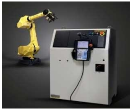
fig shows Controller unit
